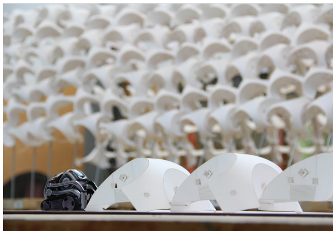
10 Robotic assembly. (Top) connecting the bricks into a chain. (Bottom) the chain in front of a final 3D mesh.
