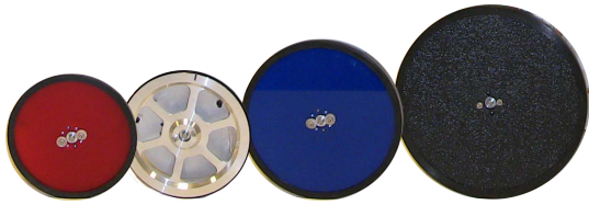
Fig. 4. We used four wheel sizes for experimental validation. These wheels are 10.16, 10.48, 12.7 and 15.24 cm in diameter.
