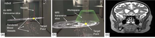
Fig. 2. (a) and (b) are holographic views that include MIR slice, blood vessel and 3D models of the robot and needle. (c) is the embedded 2D window.
