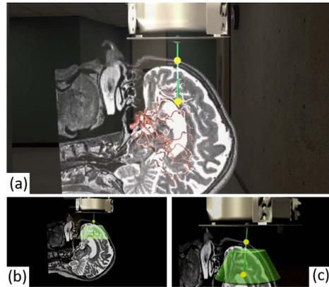
Fig. 5. HoloLens output for a case of planning with the selected target and insertion points (yellow spheres). In the different perspectives collected as the operator moves around the hologram, images, rendered vessels and the workspace can also be appreciated. The needle is colored green since its body does not collide with any forbidden zone.
