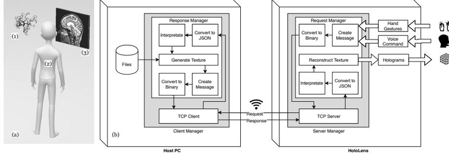
Fig. 1. (a) Topology of the holographic AR interface; the operator (1) is immersed into a scene that includes the holographic structures (2) and an embedded 2D window (3). (b) Communication of the Host PC and HoloLens.
