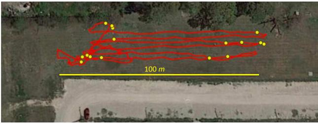
Fig. 12. Path (in red) of UAV for trial 2. Mosquito kills in yellow.
