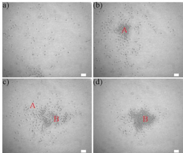
Fig 5. Building motion for swarming group of alginate microrobots. (a) Initial distribution of each alginate microrobot at 0 s, (b) The instant motion when the permanent magnet was located at 'A' position during 34 s, (c) The resultant location of alginate microrobots when the magnet was relocated the 'B' position after 45 s passed from (b), (d) The final location of all microrobots after 28 s. The scale bar represents 1 mm.
