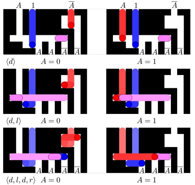
Fig. 3. A single input, two-output FAN-OUT gate. This gate requires a dual-rail input, a supply particle, and a  $2 \times 1$  slider. The *clockwise* control sequence  $\langle d, l, u, r \rangle$  duplicates the dual-rail input.
