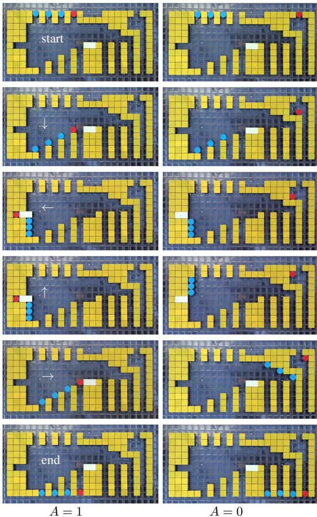
Fig. 9. Implementation of a single-input, four-output FAN-OUT gate. See video attachment at <http://youtu.be/EJSv8ny31r8>.
