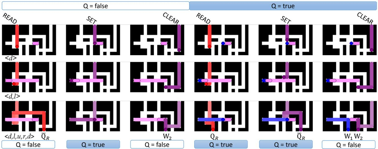
Fig. 5. A flip-flop memory. This device has three inputs, *Read*, *Set*, *Clear*, a state variable (shown in blue), and a  $2 \times 1$  slider. Depending on which input is active, the *clockwise* control sequence  $\langle d, l, u, r \rangle$  will read, set, or clear the memory.
