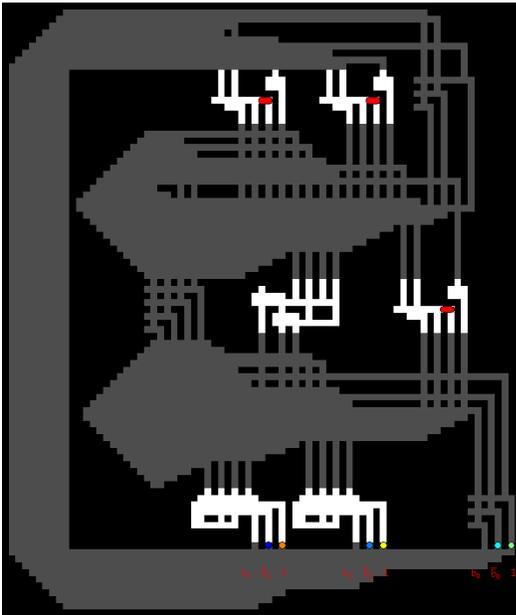
Fig. 6. A three-bit counter implemented with particles. The counter requires three FAN-OUT gates, two summers, and one carry. Six  $1 \times 1$  particles and three  $2 \times 1$  particles are used. The counter has three levels of gates actuated by CW sequence  $\langle d, l, u, r \rangle$  and requires three interconnection sequences  $\langle d, l, u, r \rangle$ , for a total of 24 moves. See video attachment for animation.
