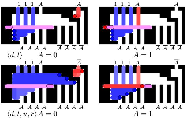
Fig. 4. The FAN-OUT gate can drive multiple outputs. Here a single input drives four outputs. This gate requires a dual-rail input, three supply particles, and a  $2 \times 1$  slider. The *clockwise* control sequence  $\langle d, l, u, r \rangle$  quadruples the dual-rail input.
