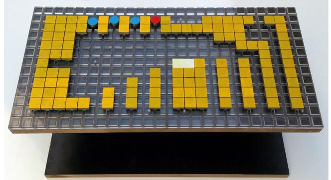
Fig. 1. Gravity-fed hardware implementation of particle computation. The reconfigurable prototype is setup as a FAN-OUT gate using a  $2\times 1$  robot (white). This paper proves that such a gate is impossible using only  $1\times 1$  robots. See the demonstrations in the video attachment <http://youtu.be/EJSv8ny31r8>.
