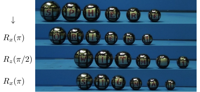
Fig. 6. Snapshots of six different-sized spheres while rolling along the three move path in Fig 5. This path consists of a roll that approximates R_x(\pi) , followed by R_z(\pi/2) , then R_x(\pi) . Four letters were printed on appropriate sides of each sphere to illustrate the movement. See the multimedia attachment for a video of this rotation sequence.
