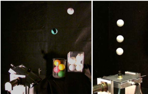
Fig. 10. Sorting multiple spheres simultaneously without camera feedback according to their ratio of drag to mass. The spheres with the highest C_d/m have equilibria higher in the jet. Left: At a flow velocity of 220 m/s, a sphere weighted to 12.9 g has an equilibrium position of 0.34 m and a sphere weighted to 6.7 g has an equilibrium of 0.49 m. By tilting the air jet, the spheres can be sorted into bins. Right: Three spheres of equal shape but differing weights are shown in equilibrium.
