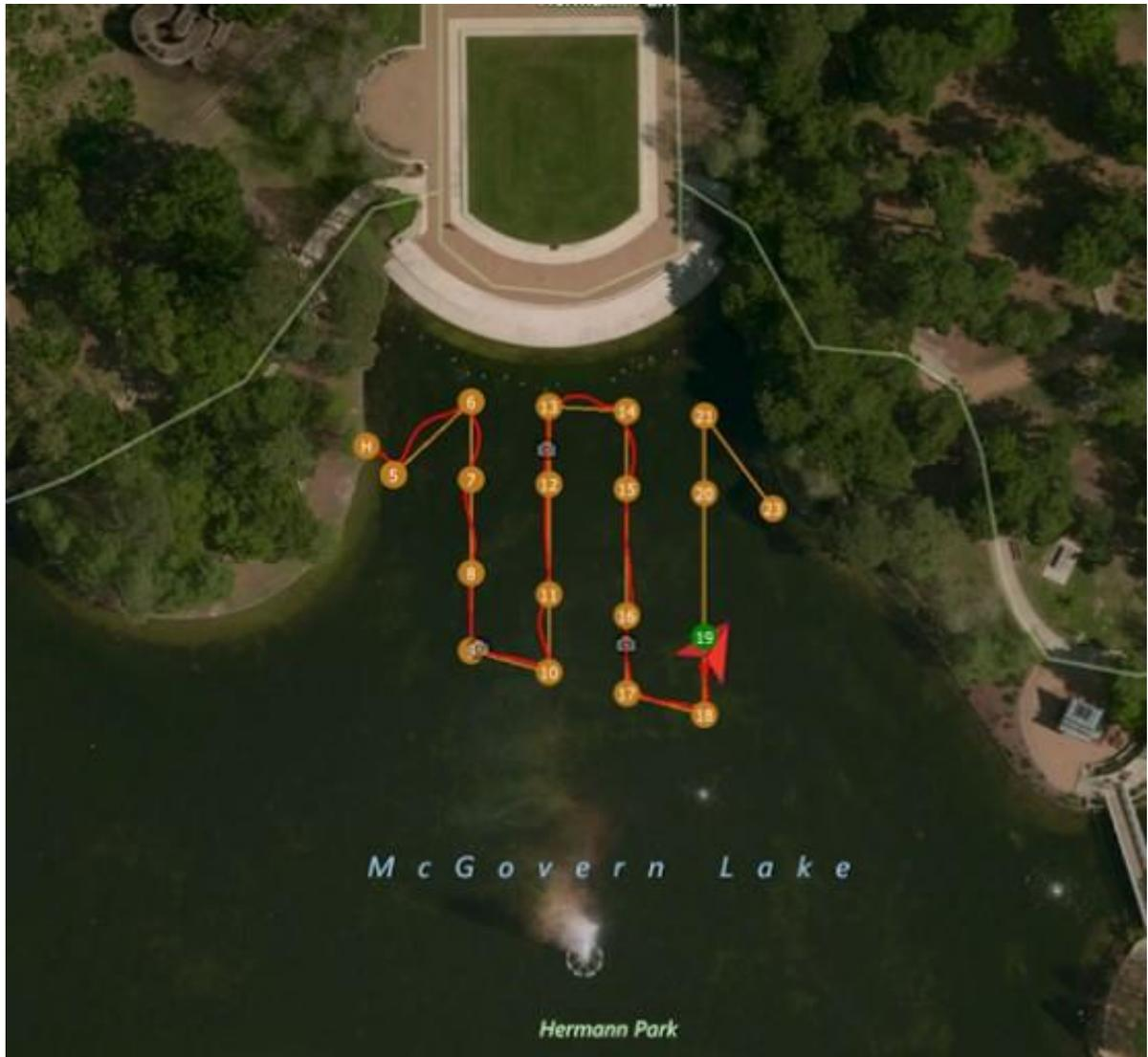
Figure 4.2: The boat was programmed to follow a boustrophedon path set by way points, which is indicated by the orange line. The red line with the arrow is the autonomous boat following the path as closely as possible.
