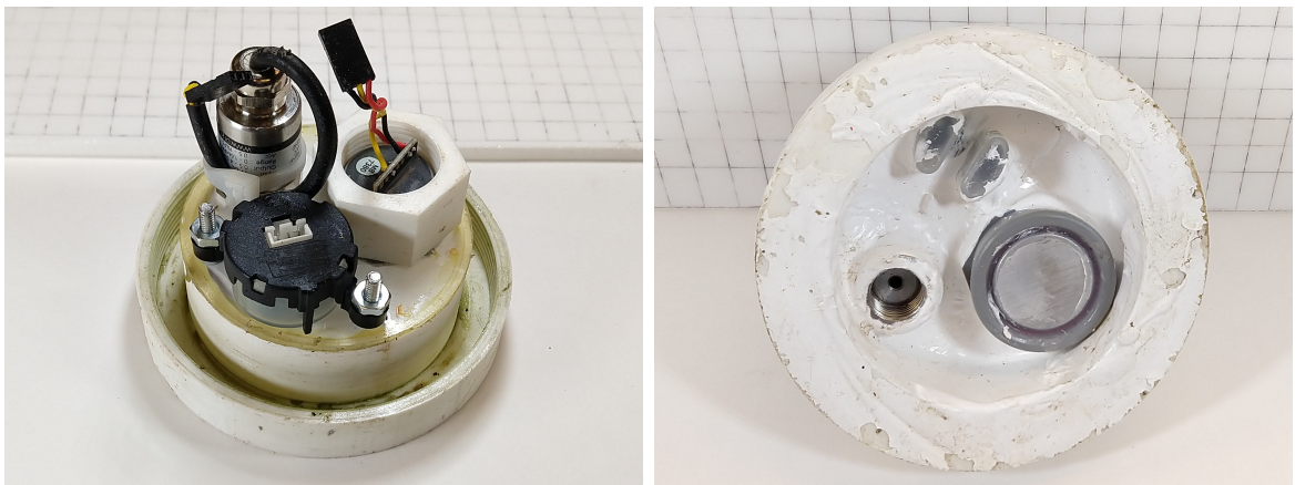
Figure 4.1: a) driftnode sensor cap. Threaded to the bottom of the driftnode. With turbidity, pressure and range sensor attached. b) bottom of driftnode sensor cap coated with rubber silicone.
