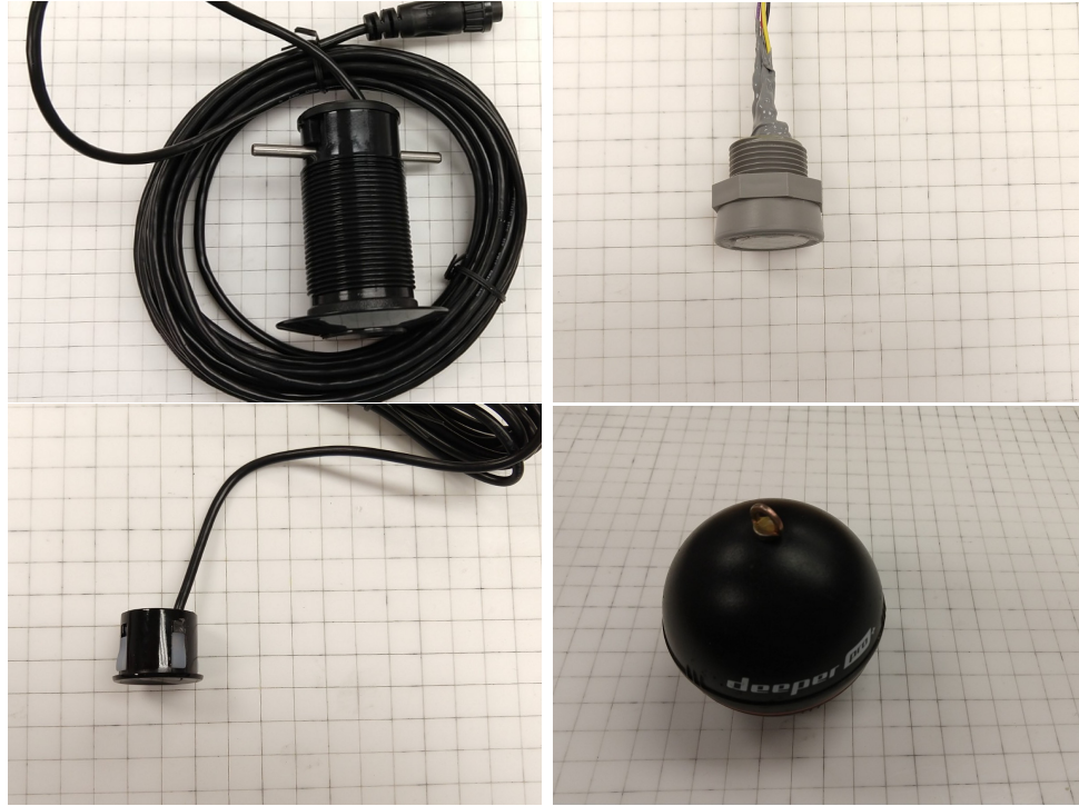
Figure 4.3: a) Garmin GDT 43 uses NMEA 2000 b) MaxBotix MB7380 use analog voltage output c) JSN-SR04T use trigger and echo timing d) Deeper Smart Sonar PRO proprietary fish finder
