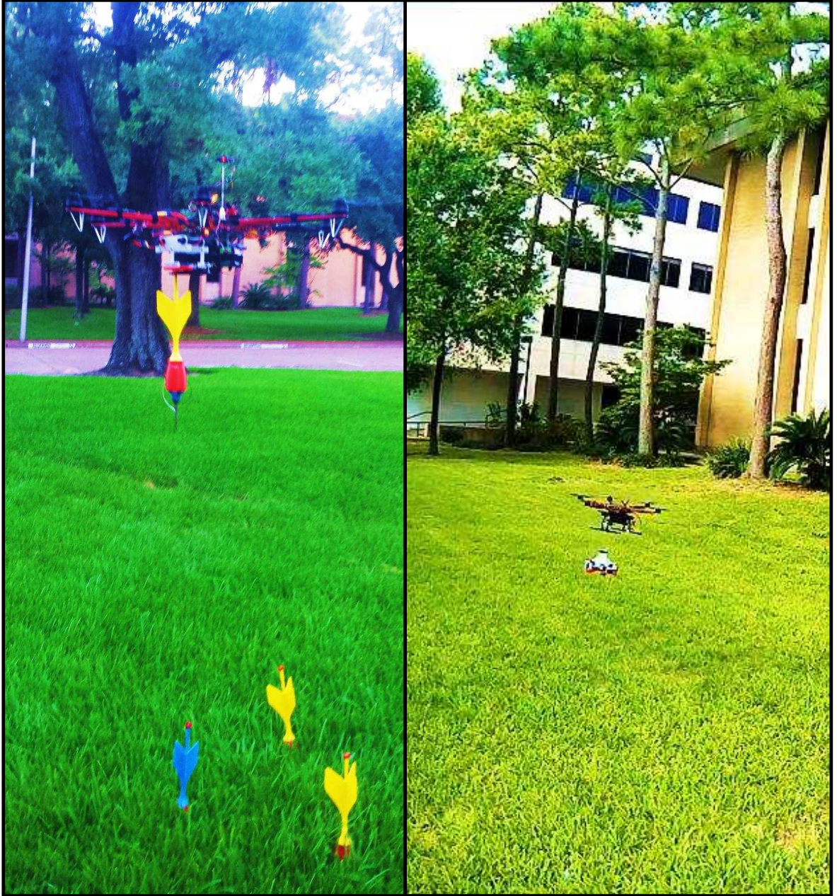
Figure 1.1: The heterogeneous sensor system presented in chapter 2: wireless Seismic-Darts and a SeismicSpider, both designed for UAV deployment.
