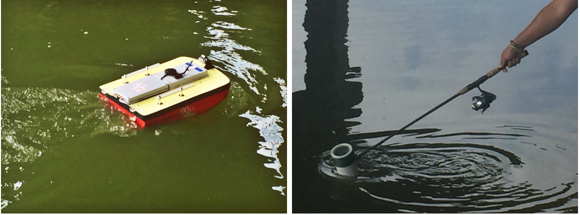
Figure 4.4: Testing the driftnode by towing the waterproof assembly behind a remote controlled boat
