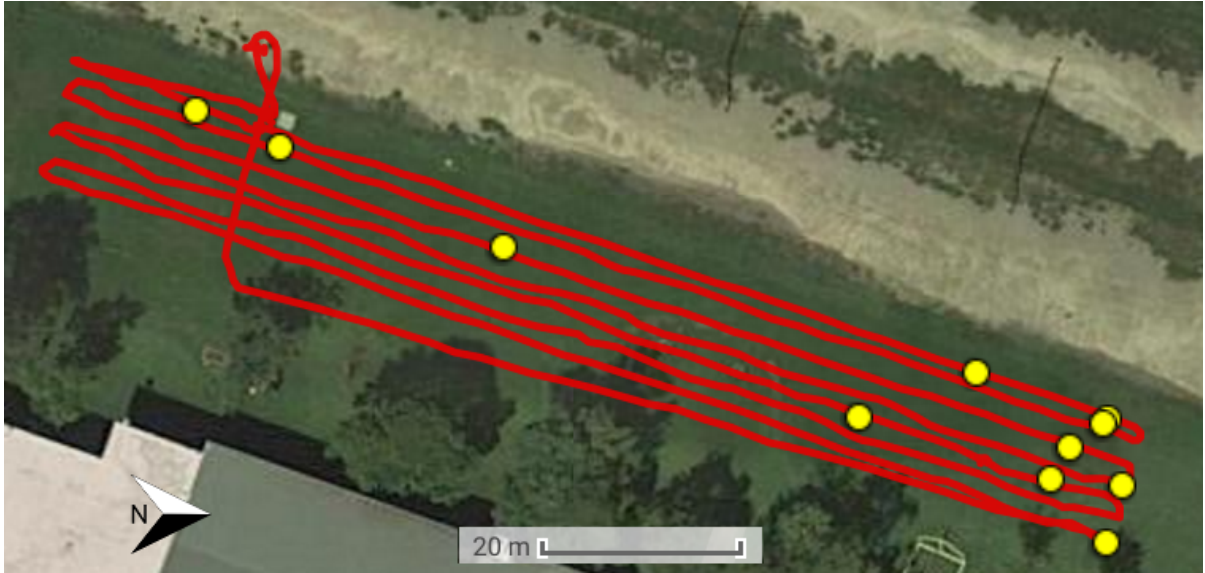
Figure 3.7: The UAV's path for flight 3 is in red. Strikes collected along this path are represented by yellow dots.
