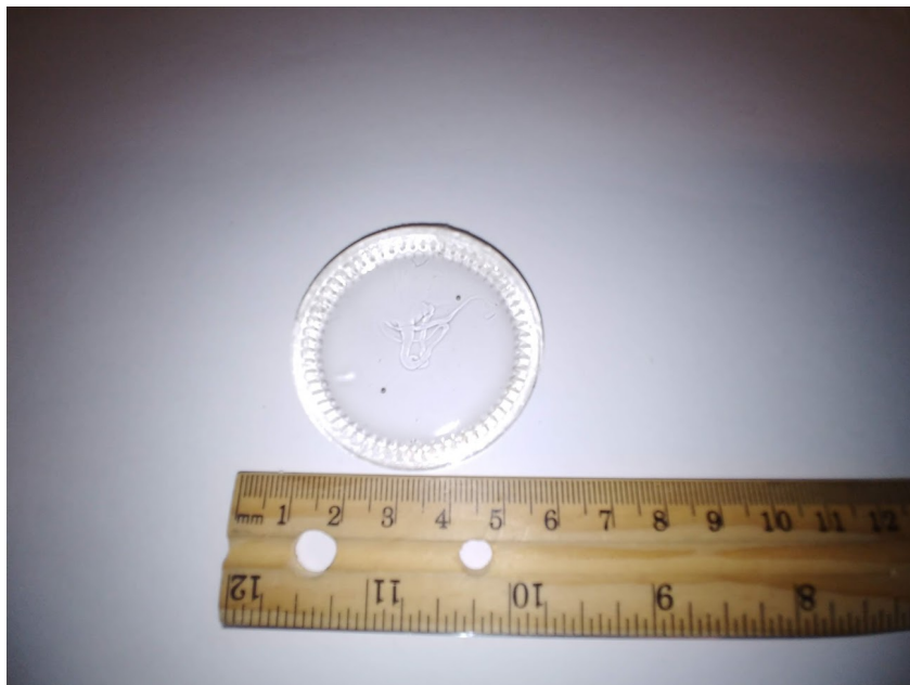
Figure 1.2: The phantom intestine model, used to simulate the small intestine of a cow along with its villi
