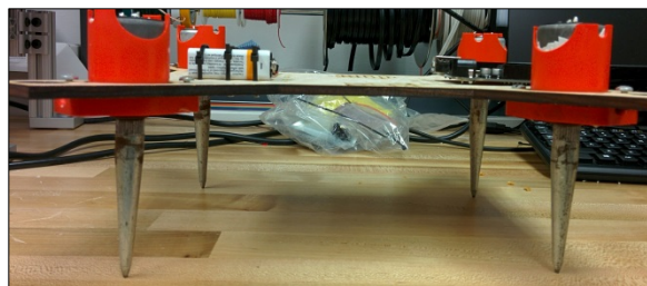
Figure 2: Design of the four-geophone platform attached to the 3DR Quadcopter.
