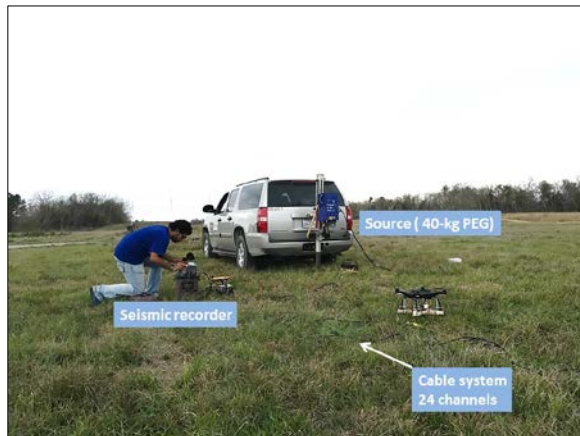
Figure 5. Field test photograph, at the La Marque Geophysical Observatory, Texas with a planted geophone and cabled system versus the drone.
